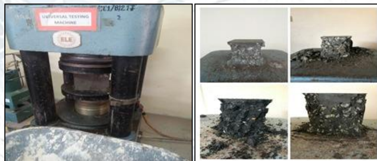
Figure 5: The concrete cube compressed by using compression machine
