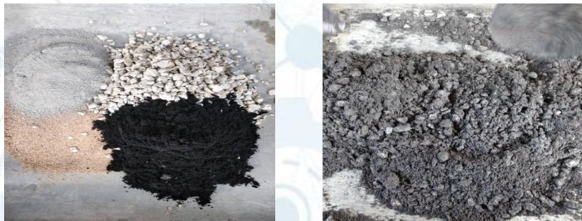
Figure 1: Mix concrete for slump test
