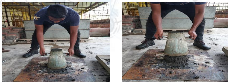
Figure 2: Compact concrete by using tamping rod
