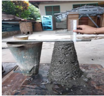
Figure 4: The slump is measured by using the upturn cone and tamping rod as a guide
